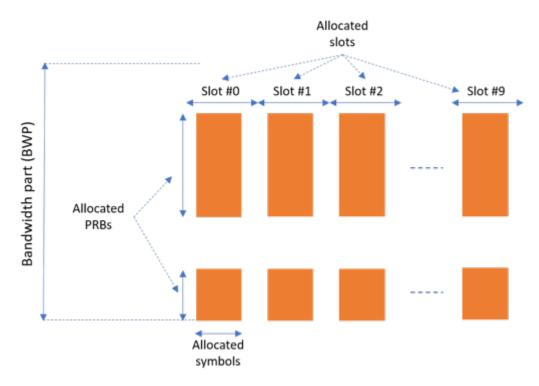
You can set the following parameters to control the PDSCH allocation. Note that these parameters are relative to the BWP. The specified PDSCH allocation will avoid the locations used for the SS burst.
