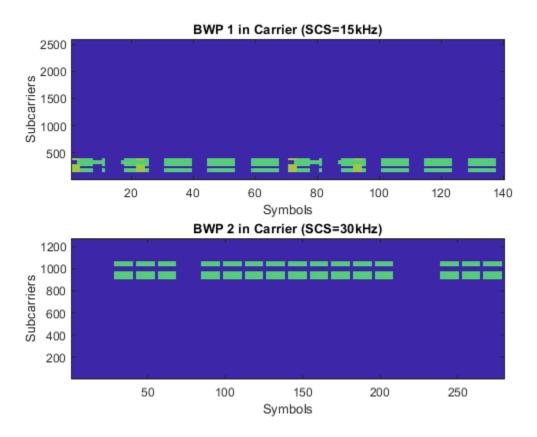
The waveform generator also plots the resource grids for the bandwidth parts (this is controlled by the field <code>DisplayGrids</code> in the carrier configuration). The following plots are generated:
